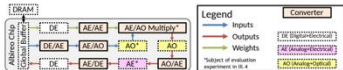
Fig. 1. Albrecht architecture. As data traverse the DE, AO, and AE domains, they leverage different movement and reuse opportunities but pay energy for data converters, notated X/Y for conversion from domain X to domain Y.
